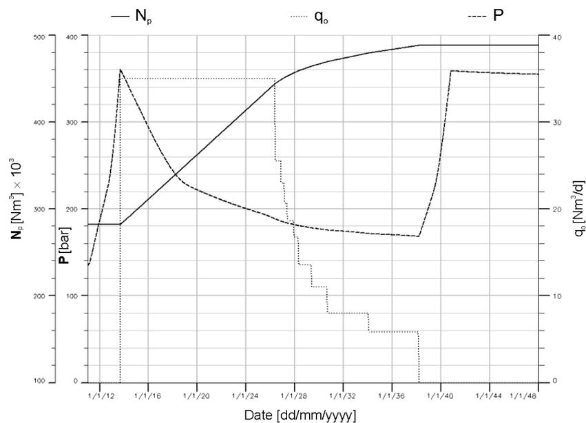
Fig. 11. Nosówka oil reservoir. Production forecast for CO<sub>2</sub> EOR. Scenario C. Total oil production,  $N_p$ , oil rate,  $q_o$ , and reservoir pressure,  $P$
