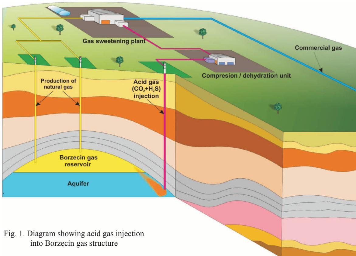
Fig. 1. Diagram showing acid gas injection into Borzęcin gas structure
