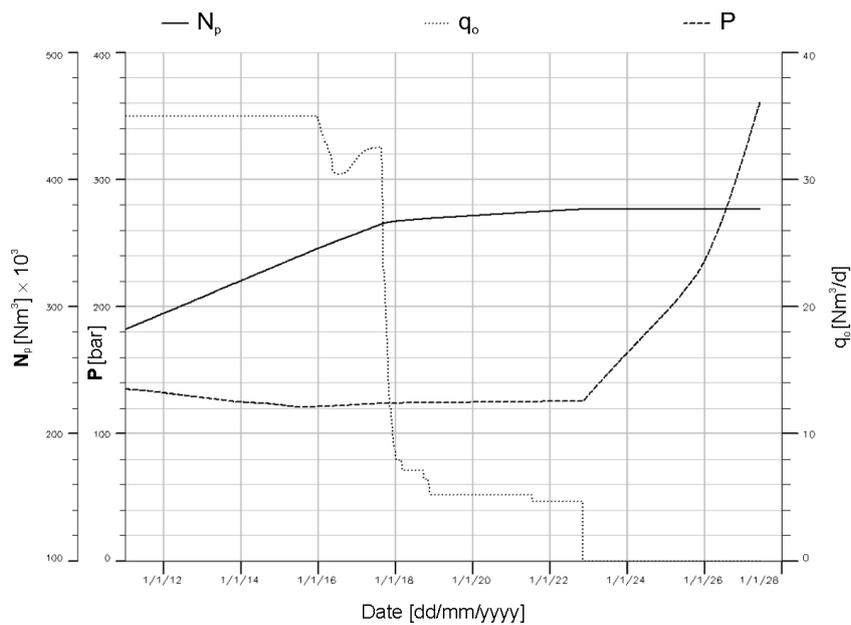
Fig. 9. Nosówka oil reservoir. Production forecast for CO<sub>2</sub> EOR. Scenario B. Total oil production,  $N_p$ , oil rate,  $q_o$ , and reservoir pressure,  $P$
