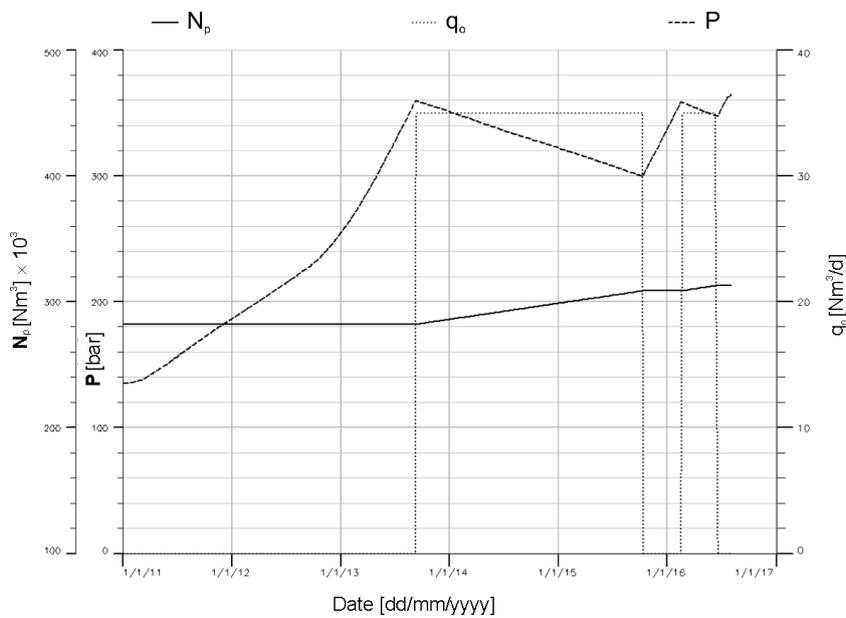
Fig. 13. Nosówka oil reservoir. Production forecast for CO<sub>2</sub> EOR. Scenario D. Total oil production,  $N_p$ , oil rate,  $q_o$ , and reservoir pressure,  $P$
