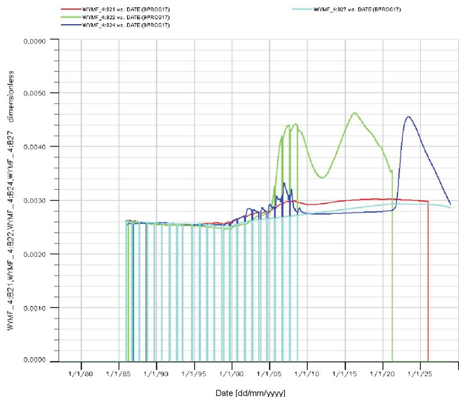
Fig. 2. Borzęcin gas reservoir. Production forecast. CO<sub>2</sub> concentration in gas wells: B-21, B-22, B-24, B-27 [5]
