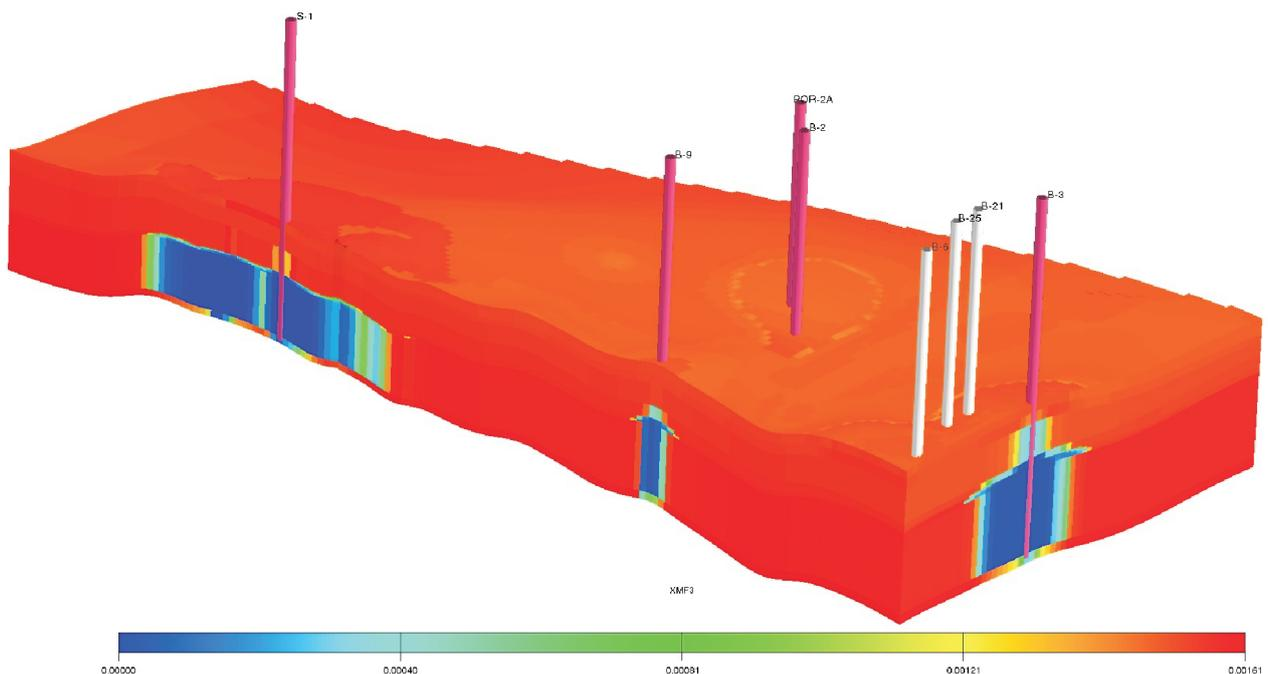
Fig. 5. Distribution of methane dissolved in brine after CO<sub>2</sub> injection into Poznań Trough Mega-structure [7]
