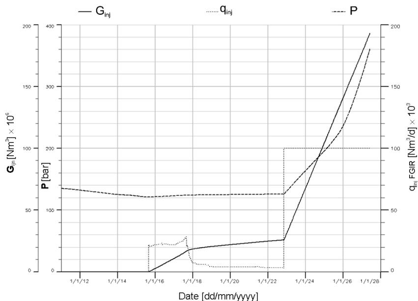
Fig. 10. Nosówka oil reservoir. Production forecast for CO<sub>2</sub> EOR. Scenario B. Total CO<sub>2</sub> injection,  $G_{inj}$ , injection rate,  $q_{inj}$ , and reservoir pressure,  $P$
