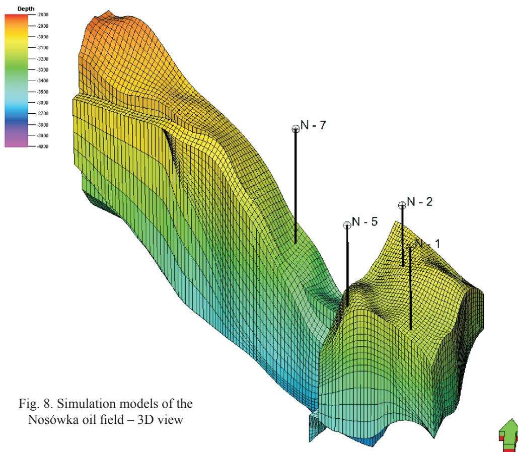
Fig. 8. Simulation models of the Nosówka oil field – 3D view
