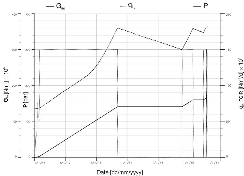
Fig. 14. Nosówka oil reservoir. Production forecast for CO<sub>2</sub> EOR. Scenario D. Total CO<sub>2</sub> injection,  $G_{inj}$ , injection rate,  $q_{inj}$ , and reservoir pressure,  $P$
