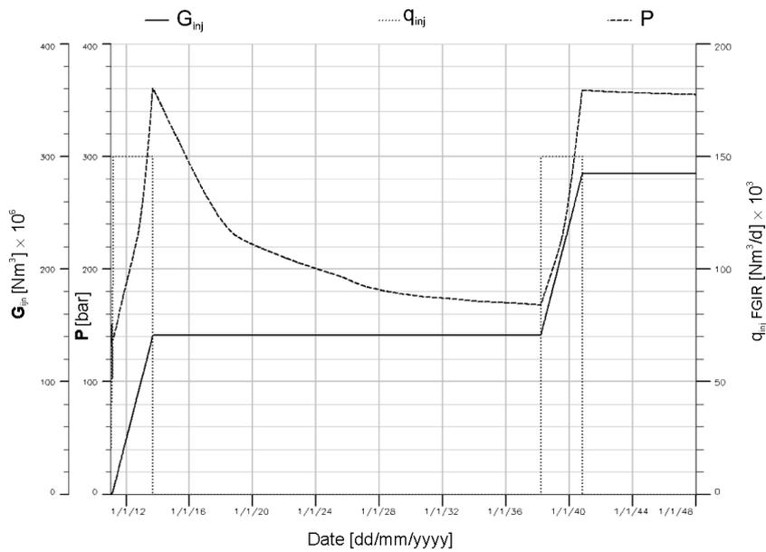
Fig. 12. Nosówka oil reservoir. Production forecast for CO<sub>2</sub> EOR. Scenario C. Total CO<sub>2</sub> injection,  $G_{inj}$ , injection rate,  $q_{inj}$ , and reservoir pressure,  $P$
