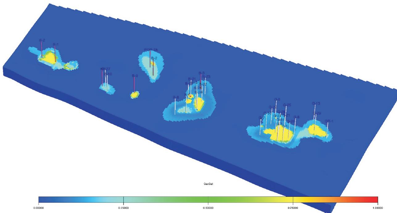
Fig. 6. Gas saturation distribution in top layers of the Rotliegend in Poznań Trough Mega-structure before CO<sub>2</sub> injection
