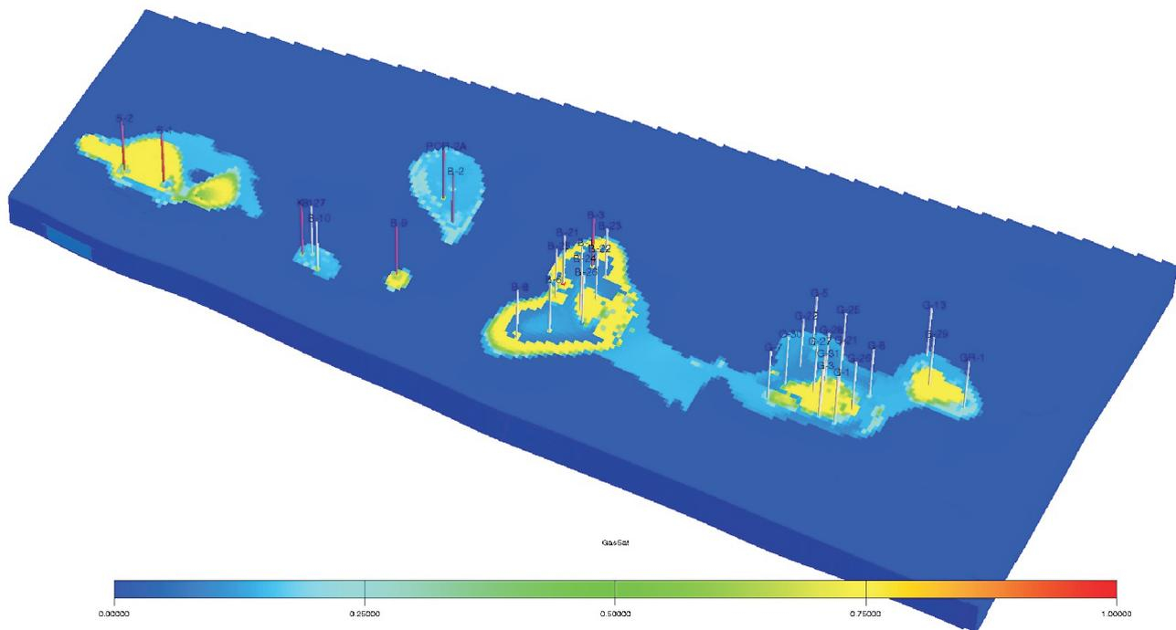
Fig. 7. Gas saturation distribution in top layers of the Rotliegend in Poznań Trough Mega-structure after CO<sub>2</sub> injection
