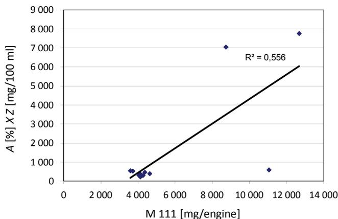
Fig. 3. Regression analysis ( $A \cdot Z$ ) versus the M 111 engine test results
