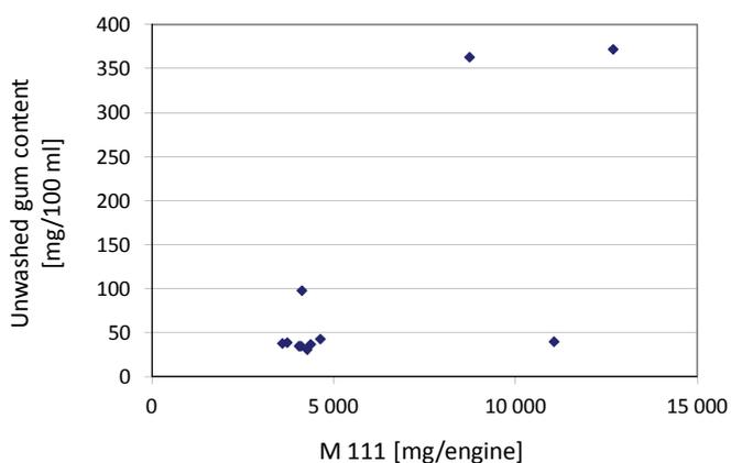
Fig. 2. Gums content ( $Z$ ) versus M 111 engine test results
