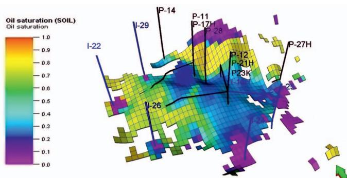
Fig. 6. Oil saturation in the selected layer of the model at the end of the production forecast (2044); Case IIA
