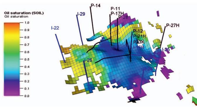
Fig. 5. Oil saturation in the selected layer of the model at the end of the production forecast (2044); Case IA
