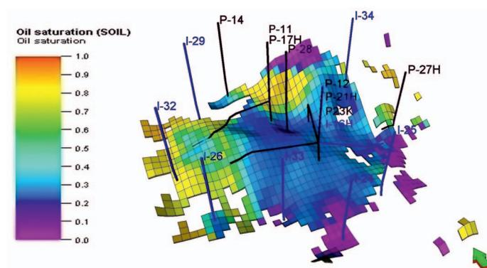
Fig. 9. Oil saturation distribution at the end of the production forecast (2044); Case IB
