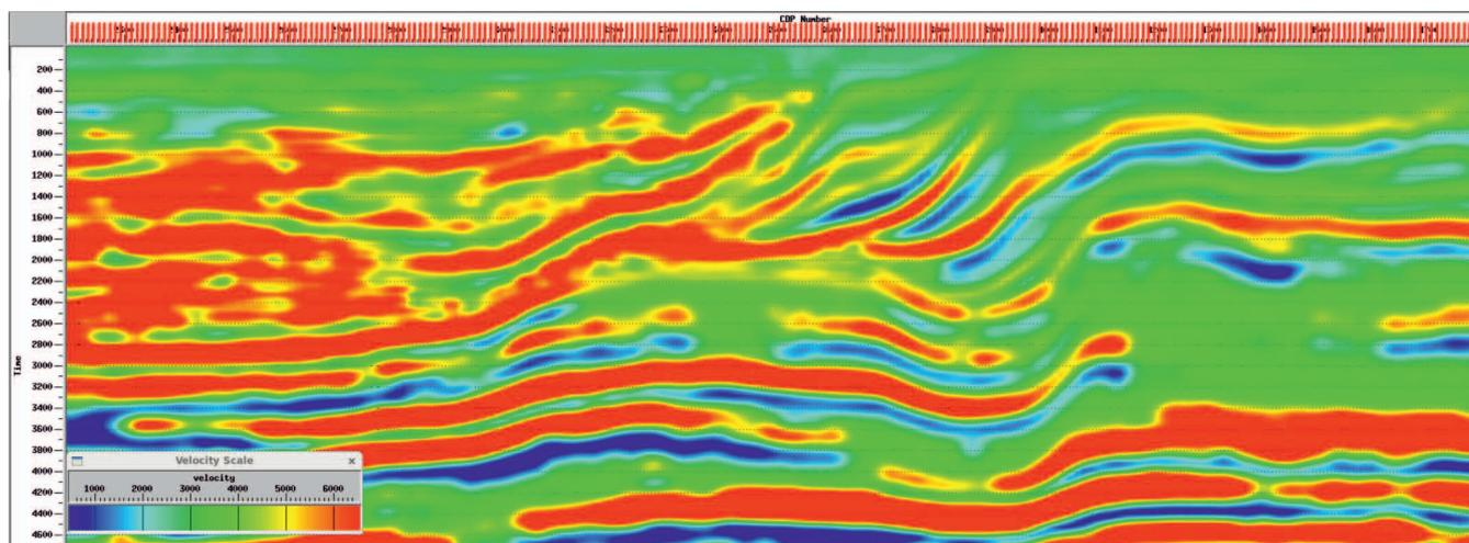
Fig. 7. Velocity model for profile no. 1 used for post-stack migration
