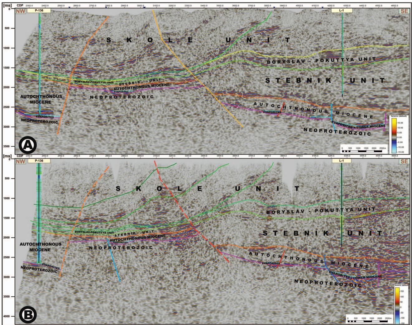
Fig. 12. Comparison of the time versions of profile no. 2: A – archival version (pre-stack); B – INiG – PIB post-processing version (post-stack)
