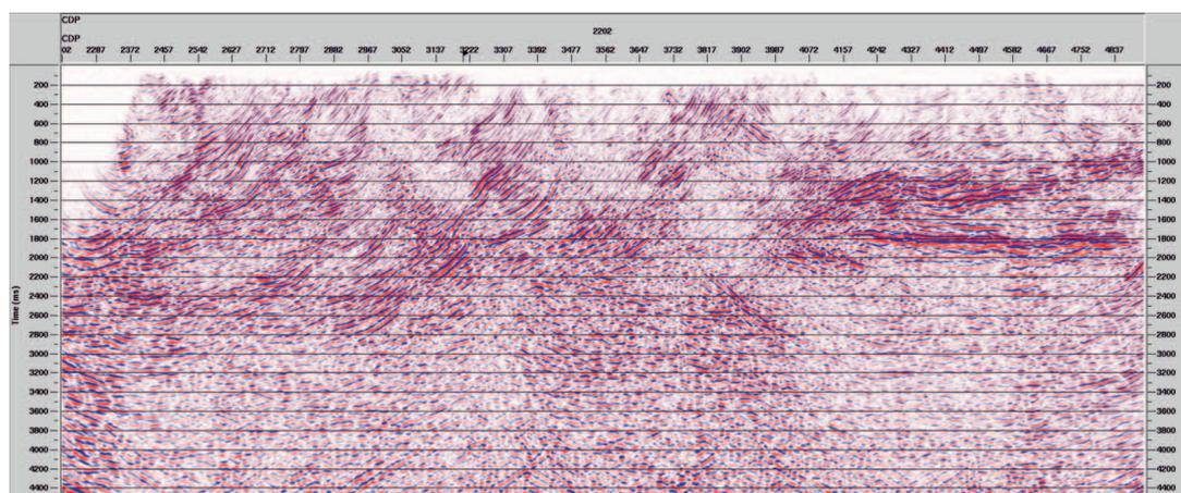
Fig. 8. Seismic section no. 1 after post-stack time migration
