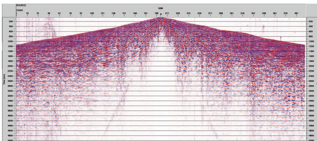
Fig. 4. Example seismic record after amplitude equalisation procedure
