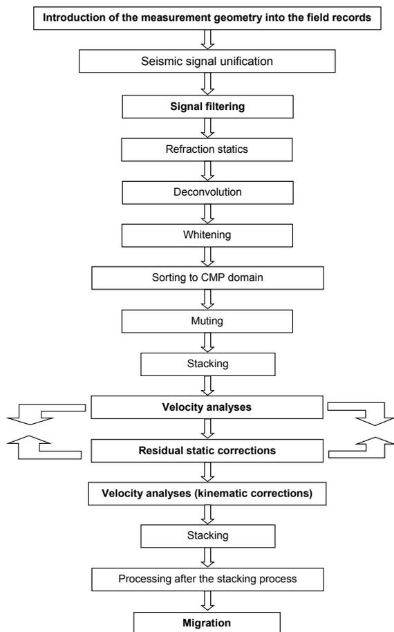
Fig. 3. Block diagram of the applied processing sequence
