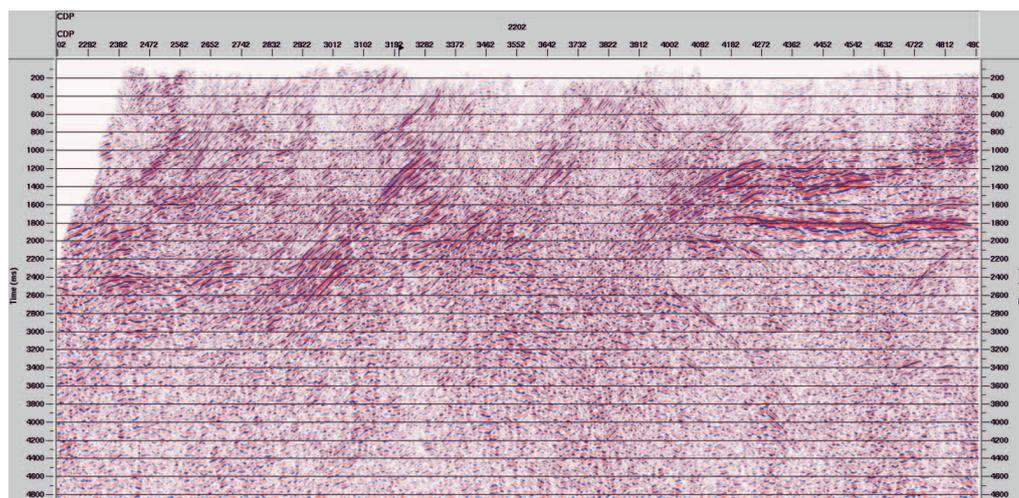
Fig. 6. Seismic section no. 1 after the stacked process
