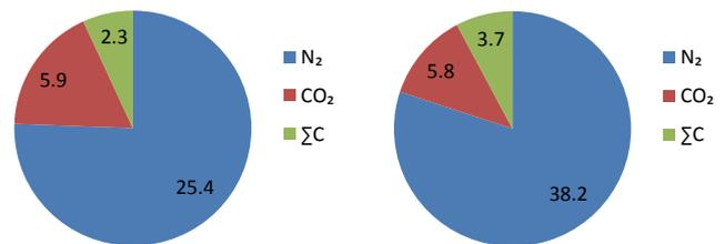
Fig. 7. Amounts of released nitrogen, carbon dioxide, and total hydrocarbons – hard coal [ml]
