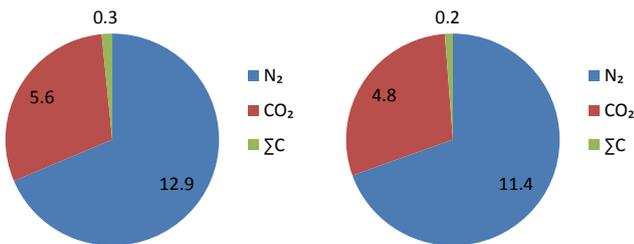
Fig. 6. Amounts of released nitrogen, carbon dioxide, and total hydrocarbons – hard coal [ml]
