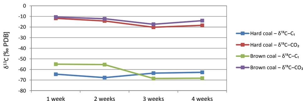
Fig. 10. Isotopic composition of carbon in methane and in carbon dioxide [‰ PDB]
