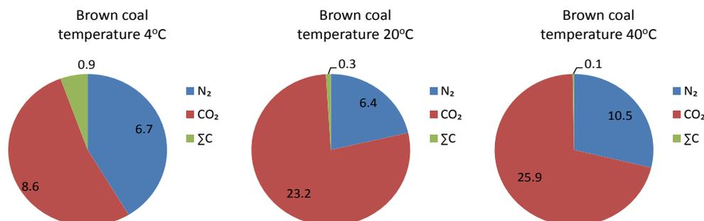
Fig. 4. Amounts of released nitrogen, carbon dioxide, and total hydrocarbons – brown coal, fraction from 0.16 to 1.4 mm [ml]
