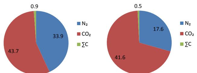
Fig. 9. Amounts of released nitrogen, carbon dioxide, and total hydrocarbons – brown coal [ml]
