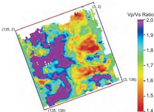
**Fig. 5.**  $V_p/V_s$  of an interval below the UMV marker at approximately 5 400 ft (1 636 m) indicating greater effective seal integrity on the west and southeast side of the study area
