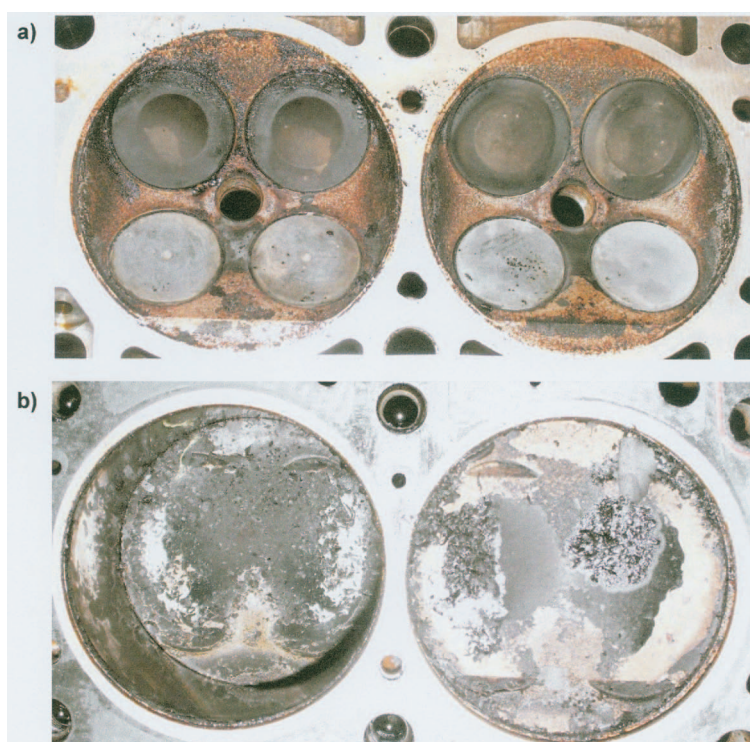
Fig. 4. Examples of deposit flaking in combustion chamber (a) and on the piston top (b)
