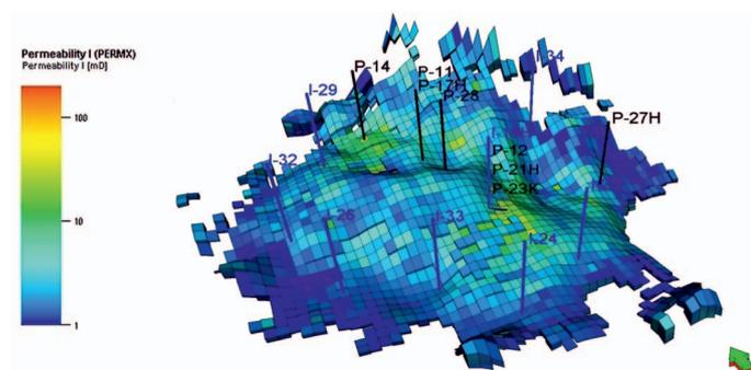
Fig. 8. Real reservoir model with additional injection wells – Base cases, IB, IIB, IIIB
