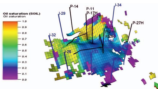
Fig. 10. Oil saturation distribution at the end of the production forecast (2044); Case IIB
