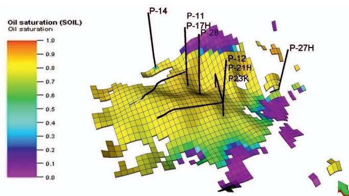
Fig. 3. Oil saturation in the selected layer of the model at the beginning of the production forecast (2017)
