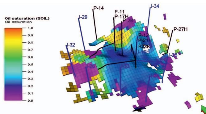
Fig. 11. Oil saturation distribution at the end of the production forecast (2044); Case IIIB
