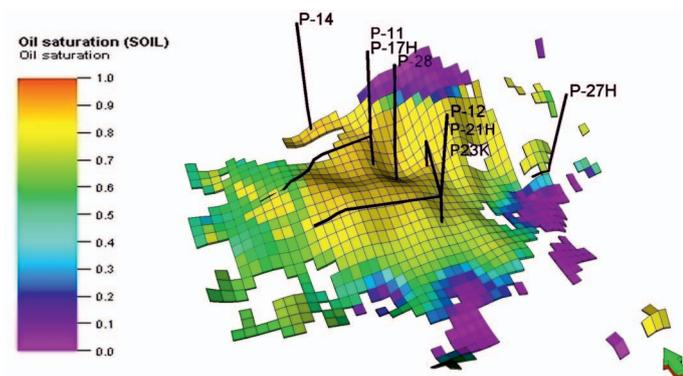
Fig. 4. Oil saturation in the selected layer of the model at the end of the production forecast (2044); Base case
